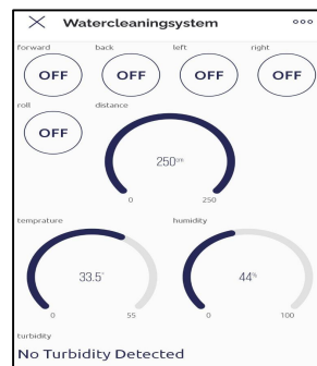
Figure 9: Ultrasonic Sensor indication in Blynk App
