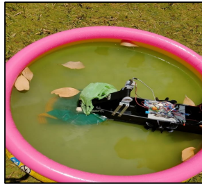
Figure 7: Collection of garbage with conveyer belt
