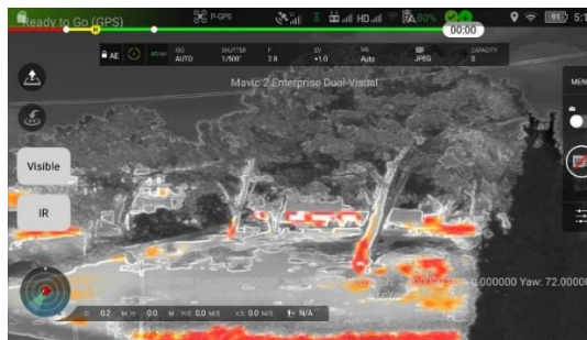
Figure 14. Ciclope drone application. DJI MSX visualization mode combining visible spectrum edge detection overlayed with the thermal image
