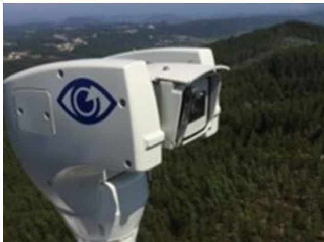
Figure 3. Motorized pan-tilt video camera
