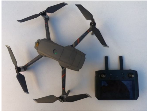
Figure 9. DJI Mavic 2E Dual and rm500 smart controller running the Android OS
