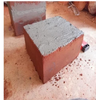
Fig 3: CSEB with application of thin layered mortar produced using granite dust
