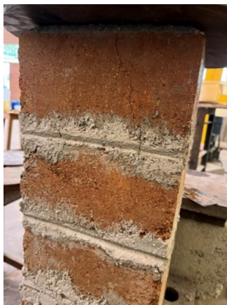
Fig 4: Typical Failed specimen under axial loading of CCM
