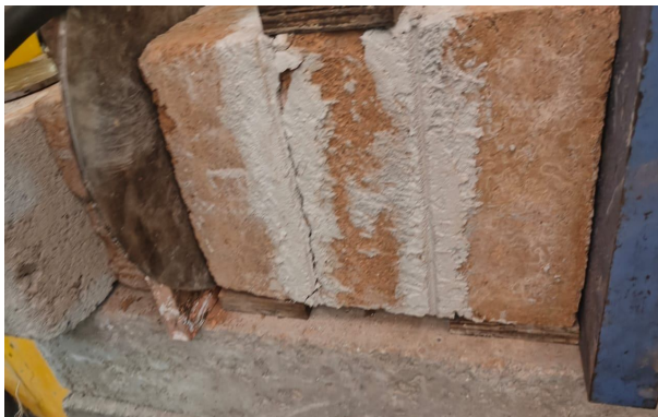
Fig 7: Typical failure pattern of CCM under shear
