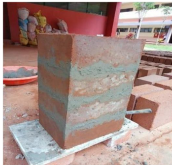
Fig 2: Typical specimen cast for masonry compressive strength test using TLM
