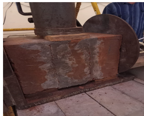
Fig 8 : Typical failure pattern of TLM under shear
