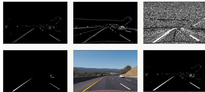
Figure 3. The images show different stages of edge detection using Sobel filtering, noise filtering, and binarization along with the raw image.
