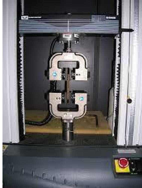
Fig. 3: Flow chart / DFD for the design process of the composite material & Machine used for tensile testing – Elastomer / UTM
