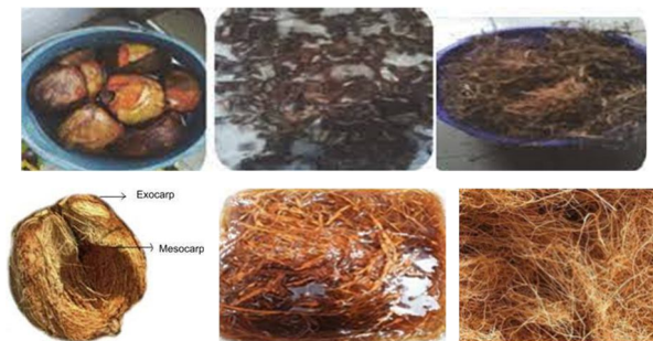
Fig. 2: General Cleaning & extraction of the coconut coil fibres – Soaked coconuts, separation of the mesocarp coirs from exocarps, soaked coco coirs, dried coirs in the sun
