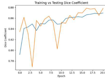
Figure 6: Dice score with ResNet-Based Encoder-Decoder model
