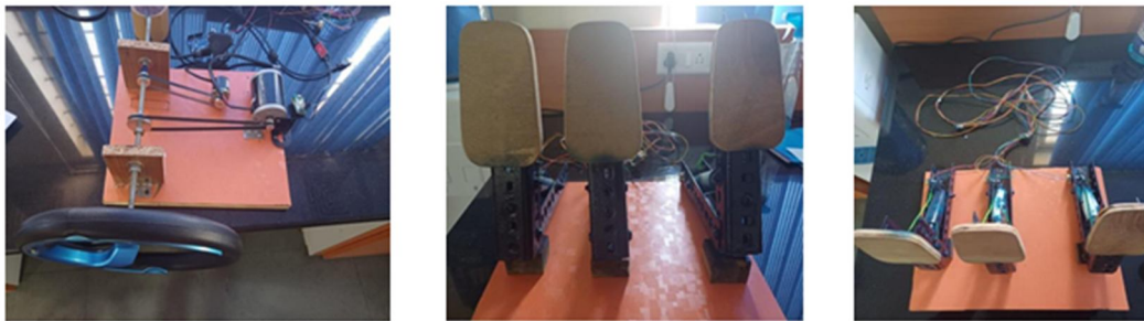
Figure 16: Pedals setup incorporating potentiometers connected to the underlying circuitry
