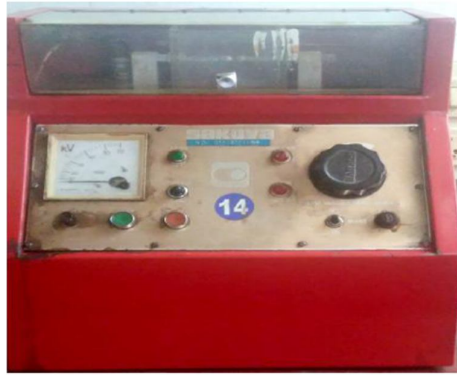
Figure 1: Experimental setup for Breakdown Voltage measurement
