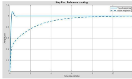
Figure 4: System response after correction(Tuner response)
