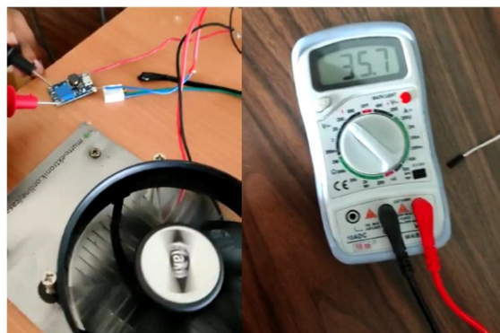
Fig. 8. Output volage generated from thermoelectric generator
