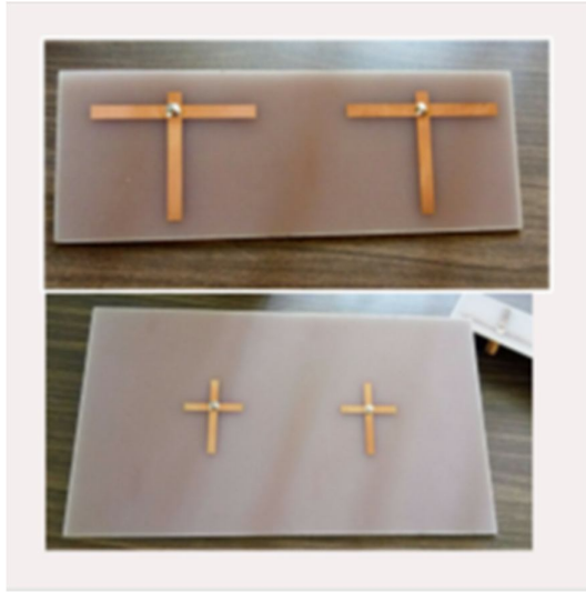
Fig. 6. Proposed MIMO antenna prototype for measurement (top view)
