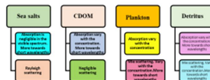
Fig.3. Absorption and Scattering Characteristics with different Seawater Compositions
