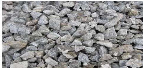
Figure 2. 20mm Size Coarse Aggregates
