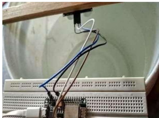
Figure.11. Ultrasonic Measurement Sensor
