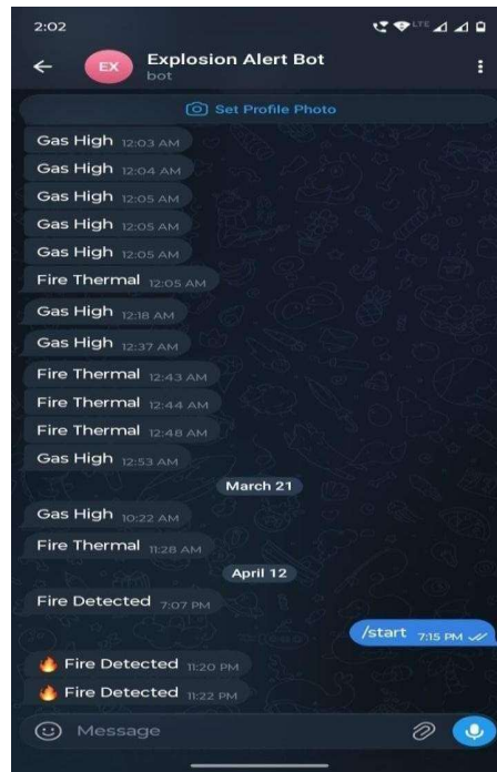
Fig 7 shows the emergency alert notification in Telegram received from the Esp8266
