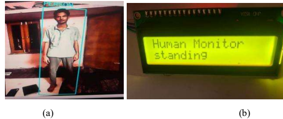
Figure. 8 Normal standing activity detection and LCD status display.
