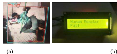
Figure 4 Fall detection and corresponding visual alert on the LCD display.
