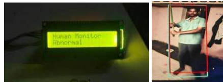
Figure 5: Abnormal behavior detection and LCD status indication.
