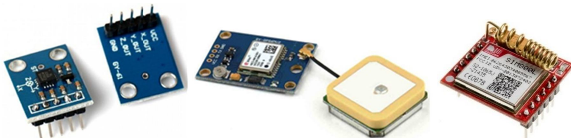
Figure 2. Pictorial representation of a ADXL335 Accelerometer, Neo 6M GPS Module & SIM800L GSM Module
