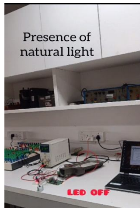
Figure.9 LED in OFF state due to the presence of natural light
