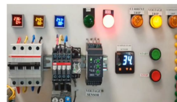
Fig 12 2: Kit after under voltage fault occurs
