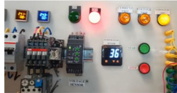
Figure 163: Kit after temperature fault occurs
