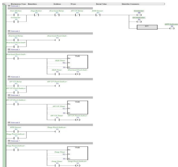
Fig 9a: Ladder program of fault detection
