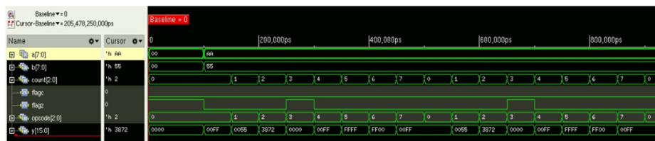
Figure 4. Simulation result of ALU in SimVision
