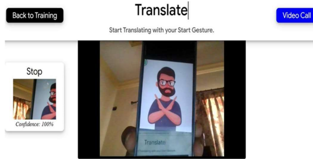
Figure 9. Final Gesture “Stop” to clear the translation and end the functioning
