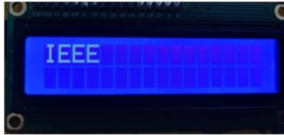
Fig. 4. Displaying Word "IEEE" on LCD Screen from Morse Code
