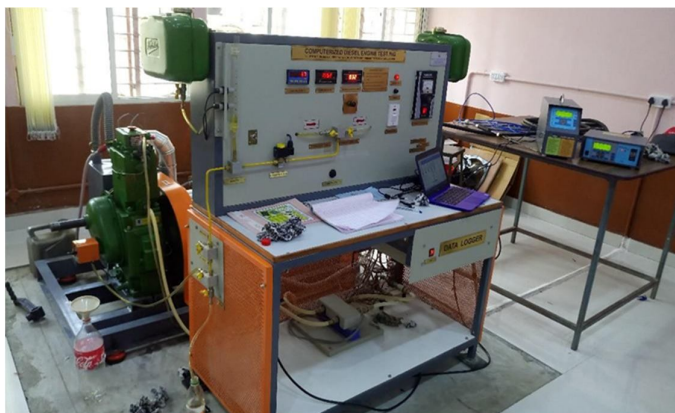
Fig. 2: Computerized Diesel Engine Test Rig
