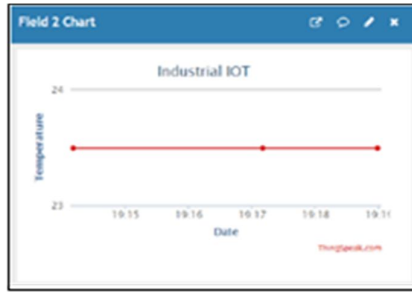
Fig.8 Thing Speak platform temperature sensor output display
