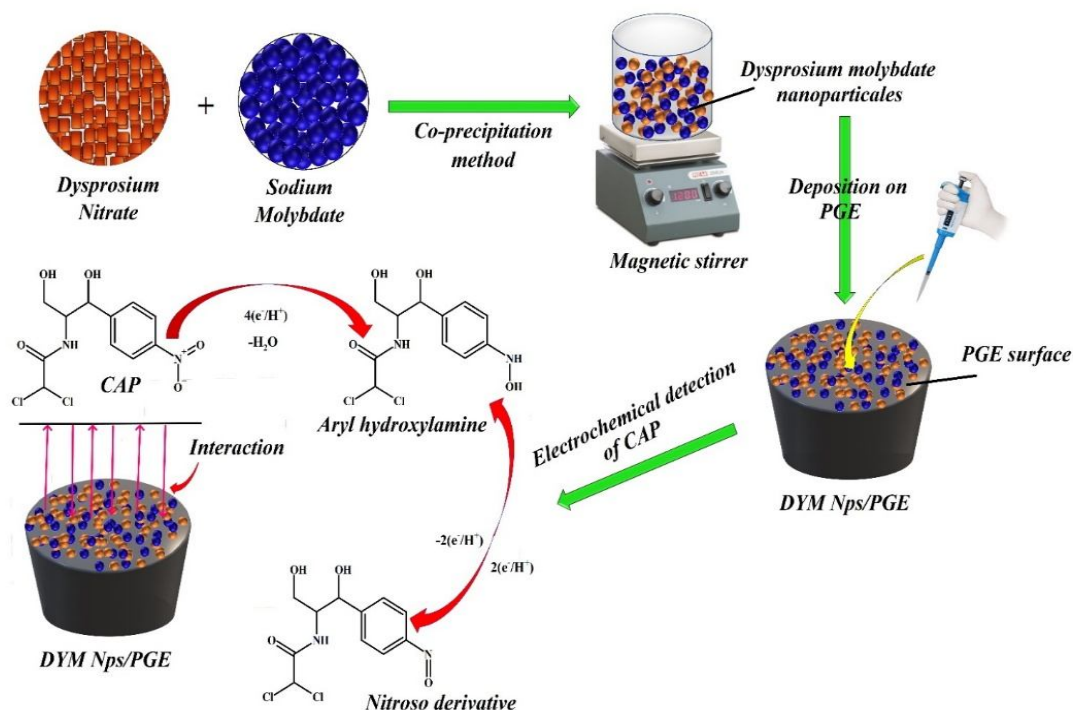
Fig 2: Schematic representation of fabrication of DYM onto the pencil graphite electrode.
