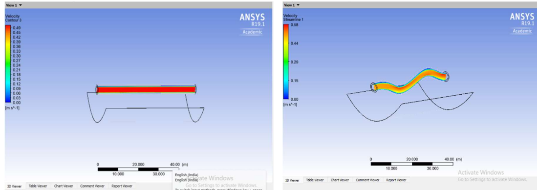
Fig.8. Velocity contour for Straight and Serpentine absorber respectively
