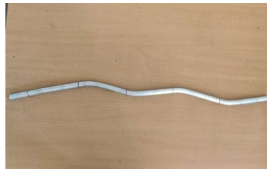
Fig.3. Serpentine Tube with Pitch 397.42 mm
