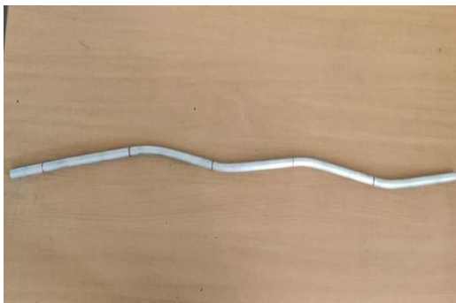
Fig.2. Serpentine Tube with Pitch 393.92 mm
