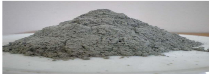
Fig 2. Sugarcane bagasse ash dumped at Sugar factory.
