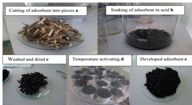
Figure 1. Process for adsorbent carbon
