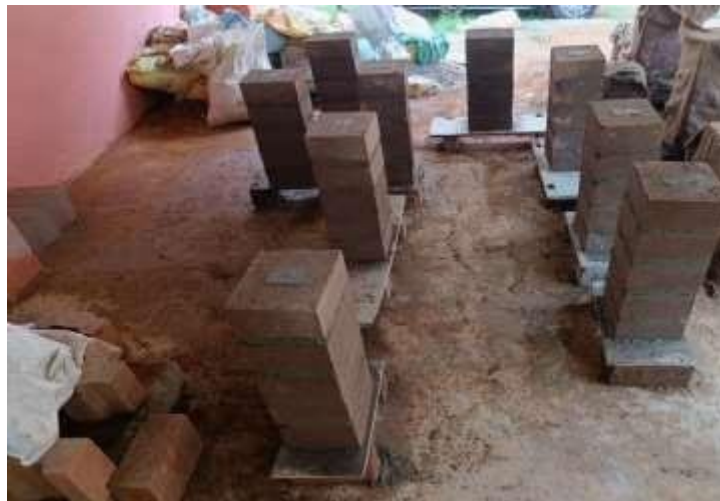
Figure 4. C and D Block prism with C and D waste mortar joints
