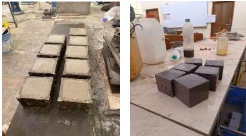
Figure 3: Casted mortar cubes and de-moulded
