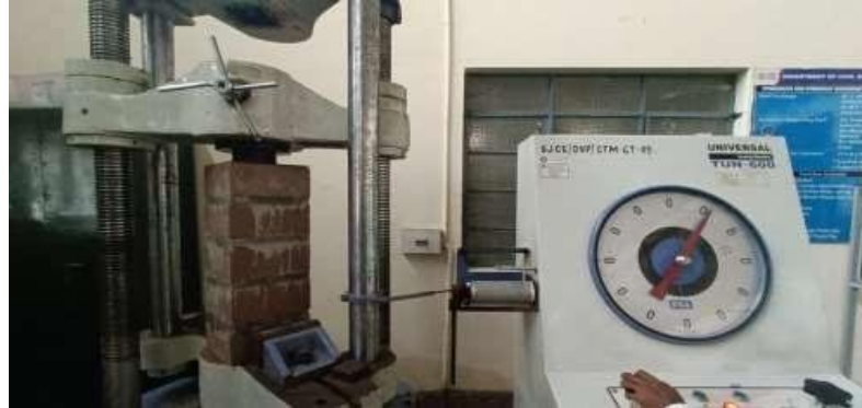
Figure 5: Test setup for the compressive strength of the prism
