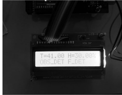
Figure 5. Snapshot of output of Fire and obstacle detected
