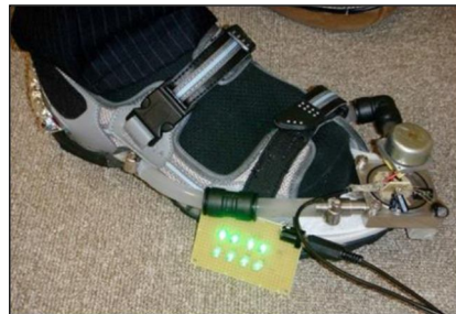
Figure 4.1 Representation of electricity generating Shoes
