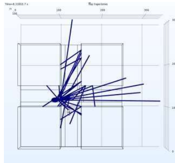
Fig 4. 3D Simulation of LiDAR at an Intersection
