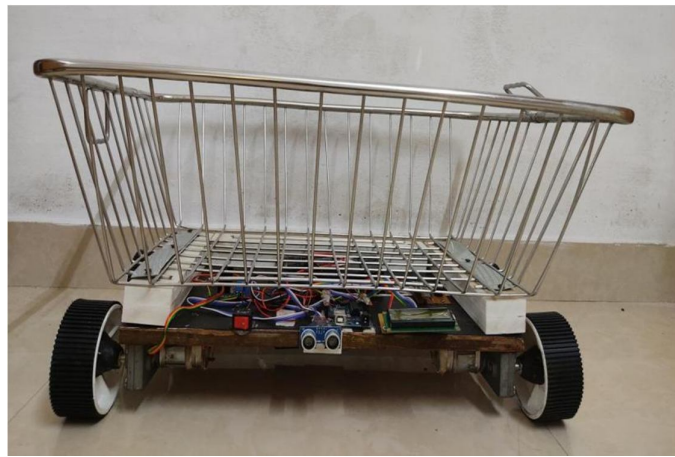
Fig. 7. Receiver section - attached in trolley
