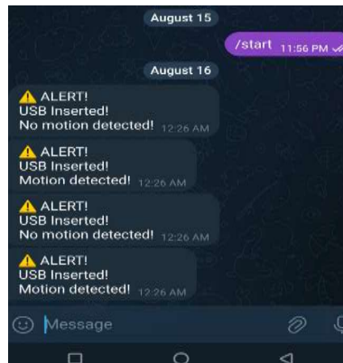
Figure 6. Telegram notification displaying real-time USB and motion detection alerts.
