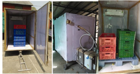
Fig. 4: A mobile cold storage facility powered by solar energy, equipped with a 0.8-tonne air
