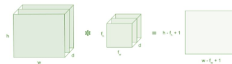
Figure9: Image matrix multiplies kernel or filter matrix
