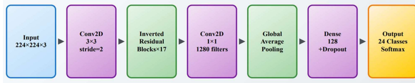
Fig. 1. MobileNetV2 architecture adapted for sign language detection. The network processes 224 \times 224 \times 3 input images through inverted residual blocks and outputs probability distributions over 24 ASL alphabet classes.
