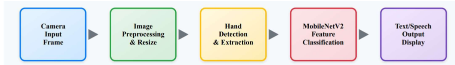
Fig. 2. Pipe line of sign language detection system. The system uses preprocessing, hand detection, classification with MobileNetV2 and gives the output as human-recognized text/speech that comes in real-time using camera input
