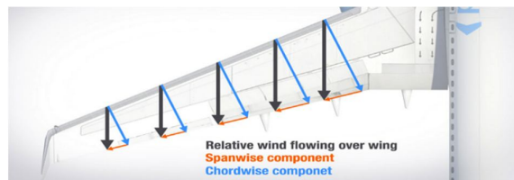
Figure 4: Swept wing spanwise flow
