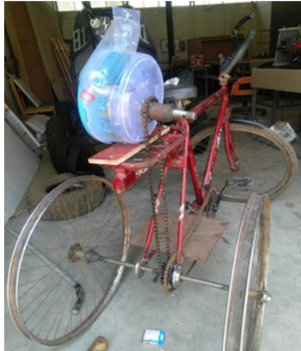
Figure 5. Actual model of pedal powered seed sowing machine
