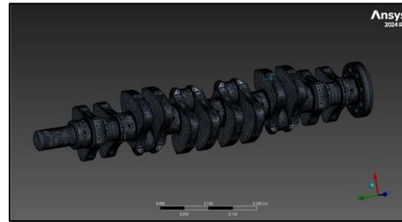
Figure 2. Finite Element Meshing of the EN24 Crankshaft
