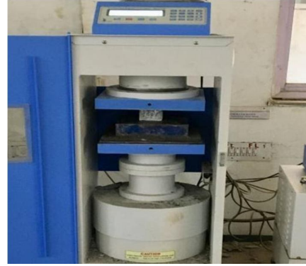
Figure 3. Compressive strength testing in Compression Testing Machine
