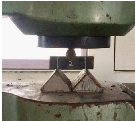
Figure 4. Testing of beam sample in Universal Testing Machine
