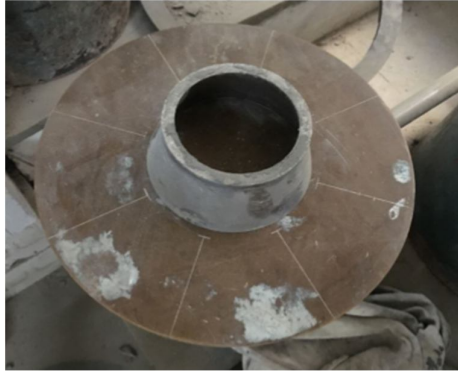
Figure 2. Flowtable Test assembly
