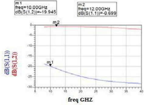
Fig 9: Return and insertion losses based on pin diode switched line phase shifter
