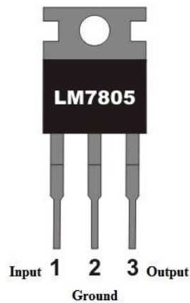
Fig. 6. Pinout of LM7805 Voltage Regulator.
