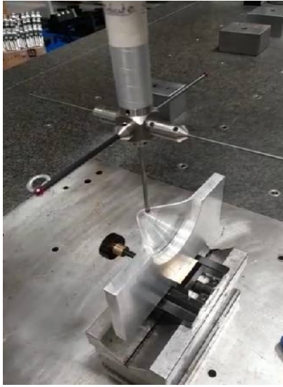
Figure 6. Thickness measurement using CMM
