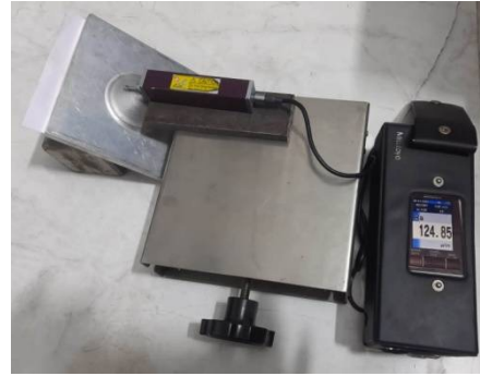
Figure 7. Surface tester measuring surface roughness
