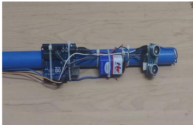
Figure 4. Working Smart Cane Stick
