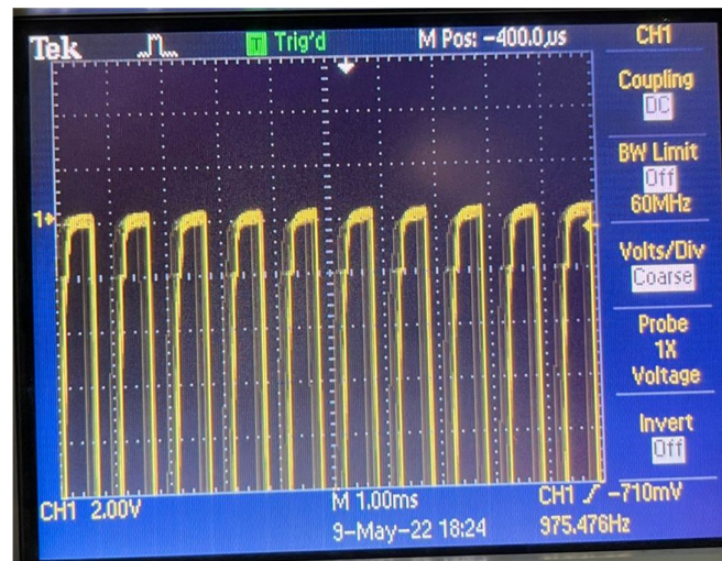
Figure 5: PWM signals of the MOSFET
