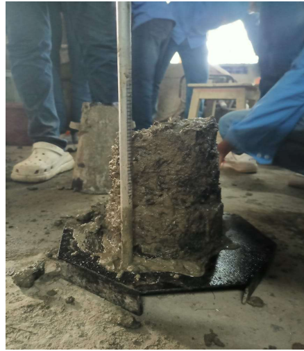
Fig 3: Slump Cone Test
