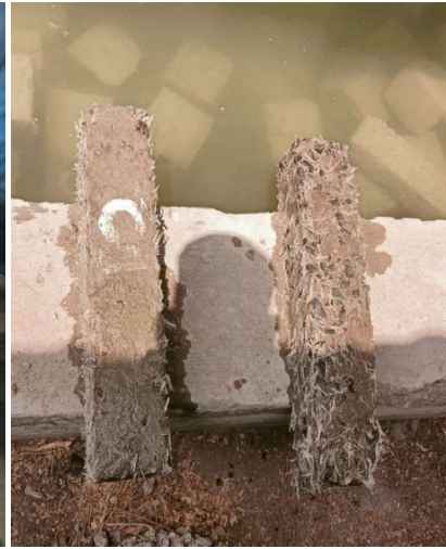
Fig 4. Casted Beam of Mixer Mixing as well as Hand mixing
