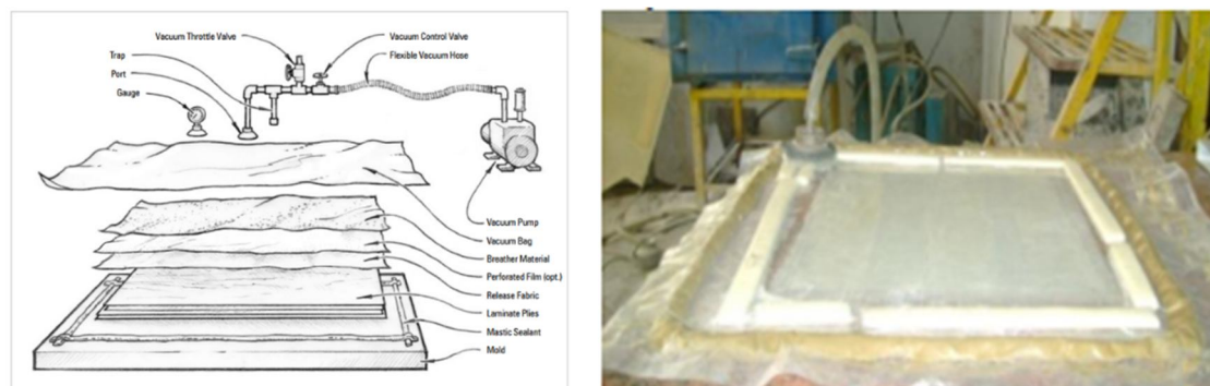
Fig 1: Vacuum Bagging Technique
