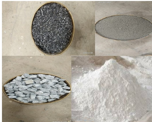
Figure 2. Materials used in preparation (Steel fibers, cement, aggregates and Metakaolin)
