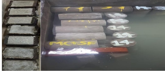
Figure 3. The samples in casting and curing
