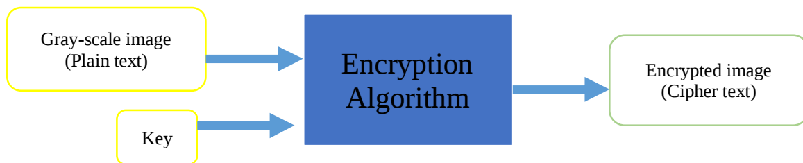
Figure 1. Generic block diagram of the encryption model
